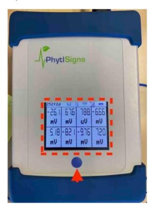
After connecting the device to the electrical grid, the PhytlSigns logo appears on the screen for a few seconds during system loading. When system loading is complete, the initial screen with the current voltage values of all 8 channels and additional information about the device is displayed:
